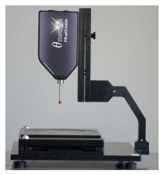
The **XY-LargePlatform** is a cost-effective solution for fast characterization of a small number of points of coatings of substrates with large footprint. The platform moves fast and manually and the user can bring under the probe any point of the substrate. It supports (upon request) reflectance and transmittance measurements.
