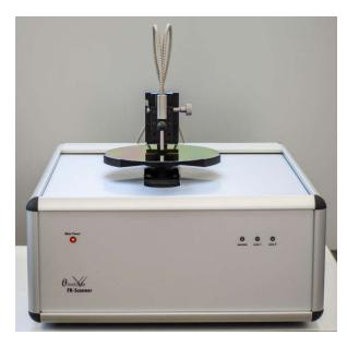
The **RO-150 stage** is a stable-top unit for the automatic characterization of coatings on wafers. It is operated through any FR-pRo unit and operates either under FR-Monitor or via the independent software that has been especially developed for daily routine use. The maximum scanning speed on 8inch wafers is 300points/min and 625measurements/90sec.
