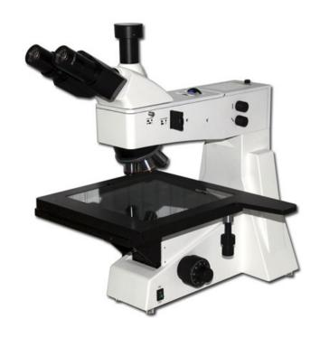
**OptiMic-200** is a top-class trinocular microscope that operate in reflectance mode and serves the characterization of coatings on wafers with diameter up to 8inch. It is ready for mounting of the FR-uProbe or FR-MicAdapter modules for the local characterization of coatings in terms of film thickness, reflectance, transmittance, refractive index.
