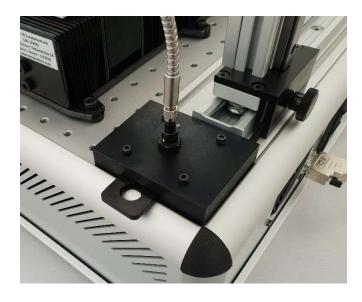
**FR-pRo-FH** can accommodate any commercially available filter of either 1/2inch or 1inch diameter. The filter can be either low-pass, high-pass or band-pass.
