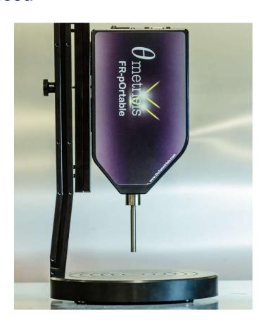
The compact size of **FR-pOrtable** along with the custom designed reflection probe, and the long lifetime (20.000h) broad-band light source guarantee highly accurate and repeatable measurements.
