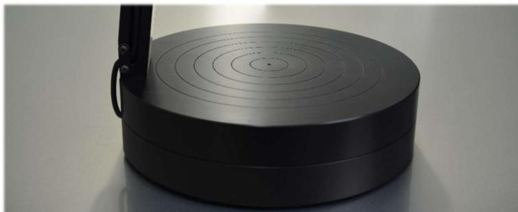
The Transmittance kit for the FR-pOrtable, is a module that is secured below the base of FR-pOrtable and is equipped with a light source similar to the one used for the reflectance measurements. The transmission light source is powered by the FR-pOrtable through the D-sub connector on the top and is controlled by the same FR-Monitor software.
