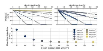
Thickness evolution during the development step corresponding to all selected exposure doses, and (top-right) only to high development rates. (bottom) The mean dissolution rates expressed as a function of e-beam exposure dose.
