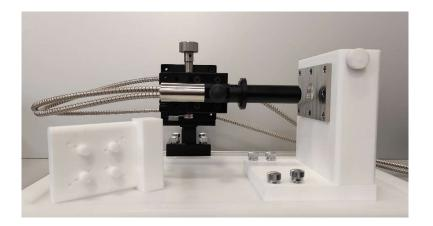
**FR-Liquid** consists of a PTFE (Teflon) cell and a holder to accommodate the sample under test. PTFE, due to its properties (hydrophobic, chemical and thermal resistant) make suitable the use of FR-Liquid for a wide range of liquids. Optical measurements with the FR-Basic tool are possible due to the optical window design on the cell, which establishes the non-contact between the optical probe and the liquid.
