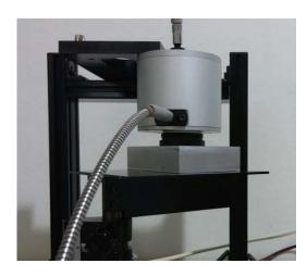
**FR-IntSphere** kit along with a FR-pRo tool is a concrete solution for reflectance measurements, without any need of additional components. The integrating sphere is made of a highly reflective, Lambertian surface (PTFE), with a sample port diameter of 10mm, compact, and easy to operate.
