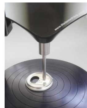
Figure 2. Specular Reflectance of the inner coating of the inside side of the press button tab of an aluminum can as recorded by FR-Monitor at left and measurement setup at right. Thickness measured at 11.4 μm .
