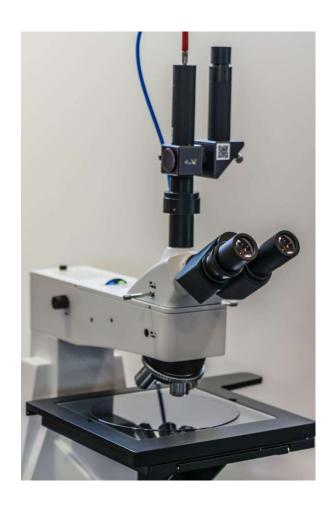
**FR-uProbe**, simply attaches to the C-mount adapter of most commercially available optical microscopes (reflectance and / or transmittance) and provides:
